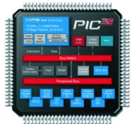
Figure 2: MC838 - PIC32 Block Diagram
